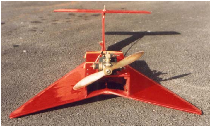
Figure 2: The MK1 Lippisch style model showing the PAR duct below the propeller
