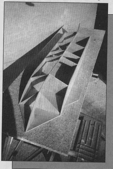
The "W" shaped lower front foil is designed to give greater roll stability at high speed than a conventional "V" shape.
